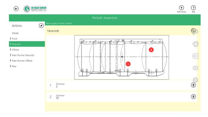
Clicking on the diagram in the Ultrasonic Thickness Test forms will place a marker and open the screen below to allow the measurement to be entered against the marker:
