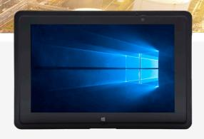
aegex10<sup>™</sup> Intrinsically Safe Tablet is certified for use in ATEX/IECEx Zone 1 and Class I Division 1 hazardous areas of industrial operations where combustible materials are present.
