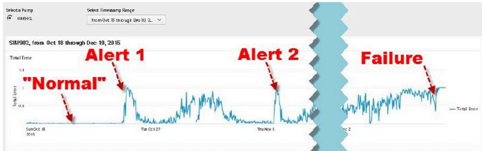
Above is a chart of Similarity's Predictive Failure Signature for the sensor data preceding the failure. After a period of normal operations, two significant alerts appear 45 and 33 days in advance of the failure. Had the customer known beforehand that this failure was looming (Alert 2), things would have been different:
