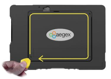
2. Use the provided pry tool to disengage the snaps. Insert the pry tool under the battery door at the bottom left corner as presented in the picture above. Then with the pry tool inserted under the door, carefully drag the pry tool around all edges and slowly lift the cover.
