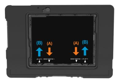
3. Release locking by pulling on the battery holder hook (A) towards the bottom of the device, then pull the battery up (B). Repeat process for other battery holder hook.
